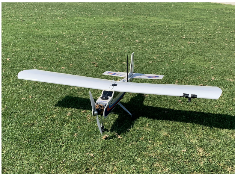
Figure 3.2: Fully assembled UAV used for practical flight tests.
