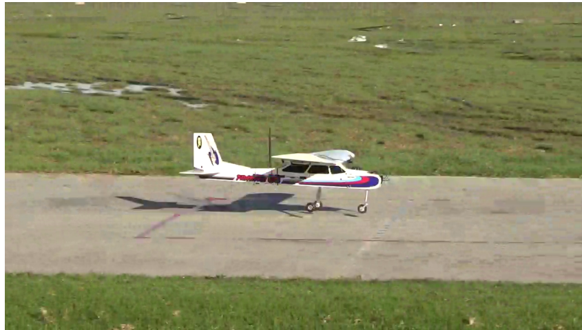
Figure 8.11: Image showing the UAV landing on the runway within the bounding box when using the classical airspeed and altitude controllers.
