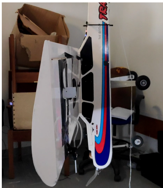
Figure A.1: Image showing the fixed-wing UAV suspended along the X-axis to calculate the I_{xx} moment of inertia.
