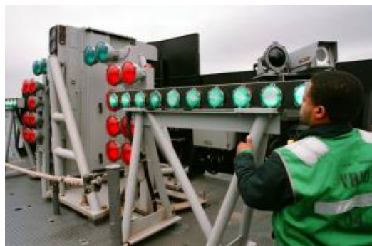
Figure 2.1: Image showing the Fresnel-lens optical landing system onboard an aircraft carrier [24].
