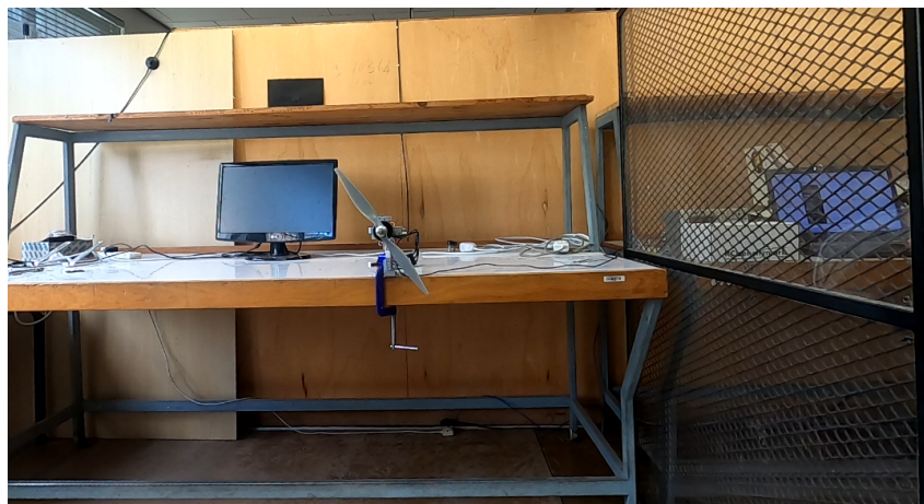
Figure A.2: Image showing the setup of the thrust jig.
