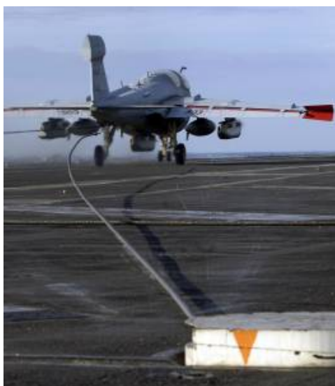
Figure 2.2: Image showing the arrestor system on an aircraft carrier slowing the fighter jet down [24].
