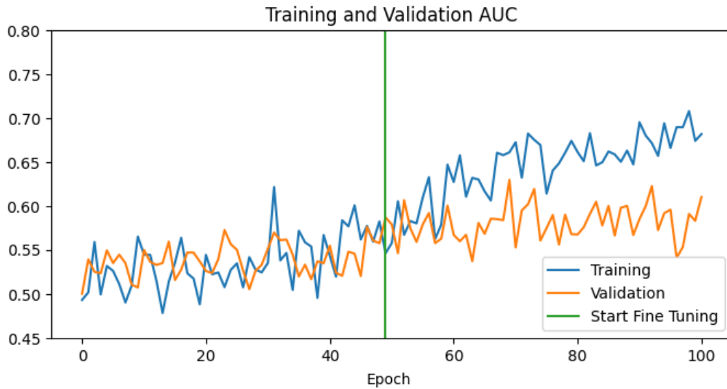
FIGURE 6.18: Visualisation of training (blue) and validation (orange) AUC curves for the training of the prediction model where the initiation of unfreezing two convolutional base layers are indicated with the green vertical line.
