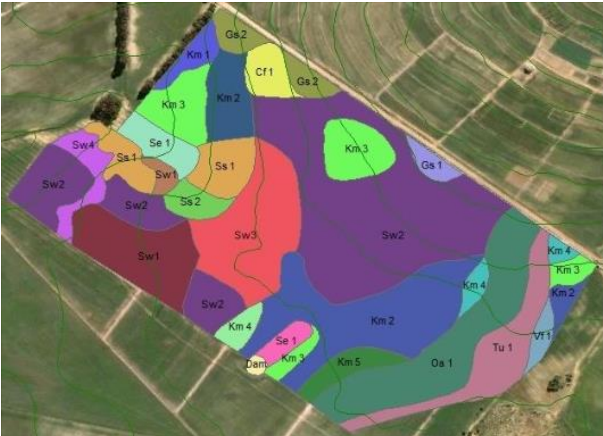
Figure 10: A soil map of the study site at Langgewens Research farm, Western Cape, South Africa. The soil form are Swartland (Sw), Klapmuts (Km), Cartref (Cf), Glenrosa (Gs), Oakleaf (Oa), Sepane (Se), Sterkspruit (Ss), Tukulu (Tu), and Vilafontes (Vf) (Ellis, 2010)
