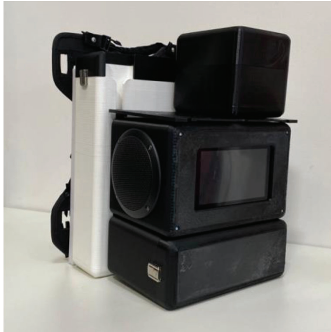
Figure 53: Prototype of modular intelligent mobility box (Kunz, 2022, p. 64).
