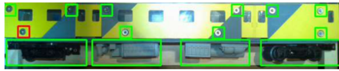
FIGURE 6.13: System detects that one part is missing [27]
