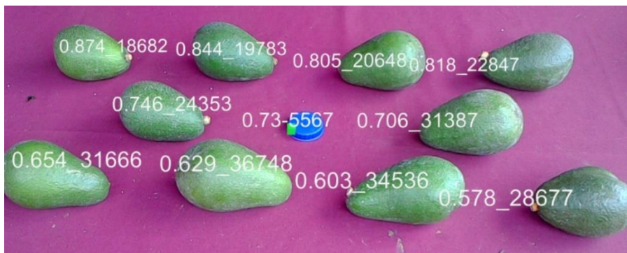
Figure 5.6: Figure of a photo taken from the HoloLens during development which shows the distance to the HoloLens and the number of pixels contained within each avocado in the HoloLens’ field of vision
