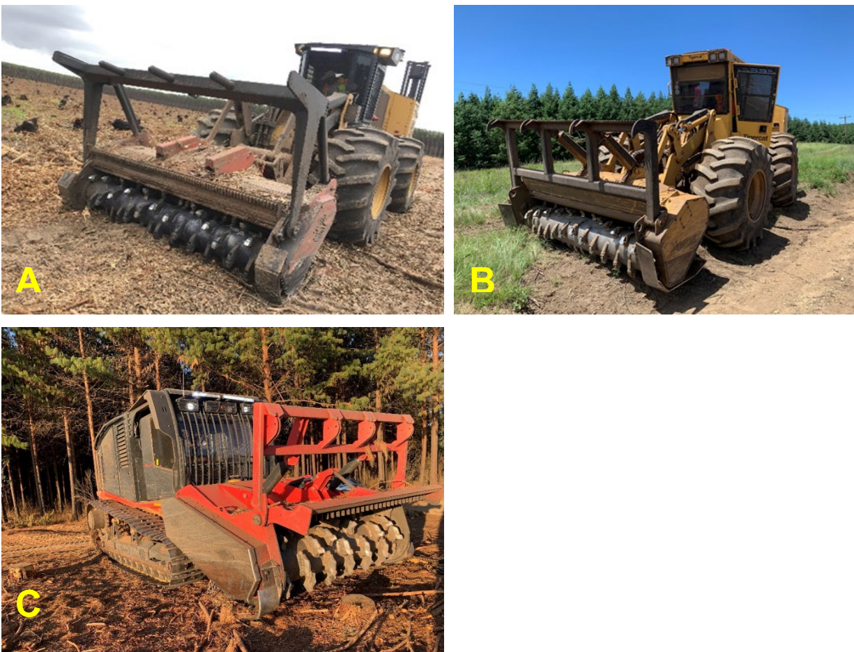
Figure 3.13 Horizontal drum mulching machine investigated, A- Cat 586C base machine with a FAE 300U mulching head. B- Tigercat M726G mulcher. C- Prinoth Raptor 800 mulcher.
