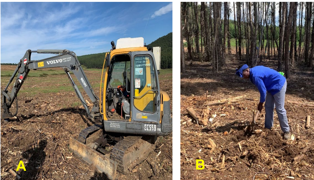
Figure 3.15 Pitting methods, A- Mechanised Mpat single pit pitting machine. B- Manual pitter equipped with a Pick.
