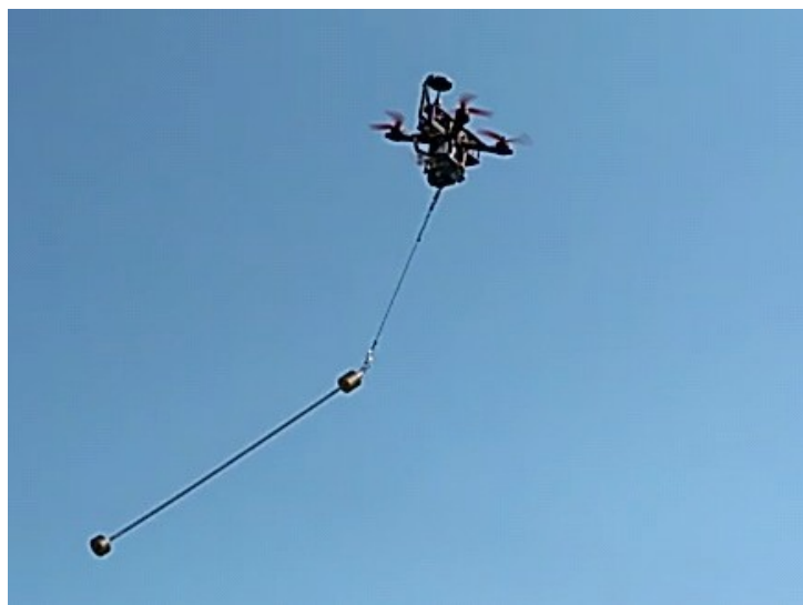
Figure 7.4: Practical flight with a suspended elongated payload attached to Honeybee.
