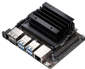
Figure 6.4: NVIDIA ® Jetson Nano ™ [9] used as a OBC.
