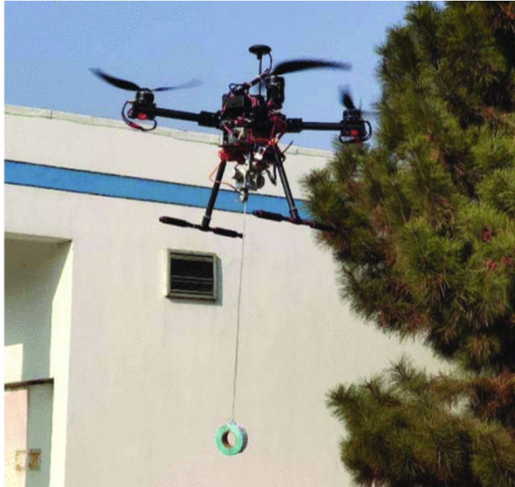
Figure 2.5: Multirotor and suspended payload for outdoor experiments [4].
