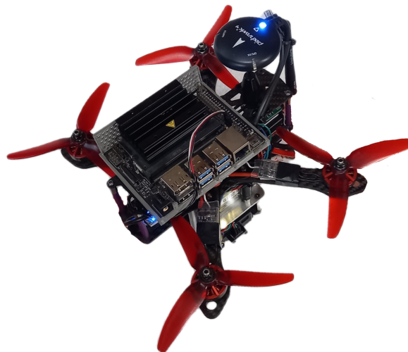
Figure 6.1: Honeybee multirotor equipped with a OBC and payload angle sensor.
