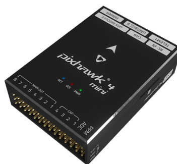
Figure 6.2: Photo of a Pixhawk 4 mini FC [7].
