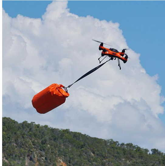
Figure 2.2: A practical suspended payload used for search and rescue missions [1].
