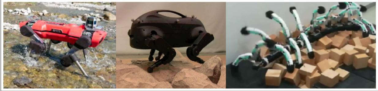
**Figure 2.7:** The robots that tested the different approaches to overcoming rough terrain. ETH Zurich AnyMAL on the left, the littleDog in the middle and the Shinayaka robot on the right.
