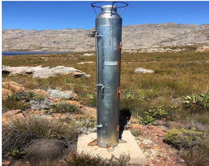
Figure 9: Hellmann rain gauge used to measure rainfall at Olifants Doorn.
