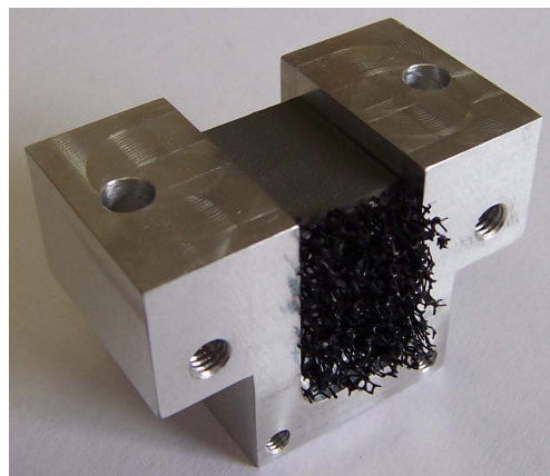
(d) Positions of resistive sheet and reticulated foam absorbers.
