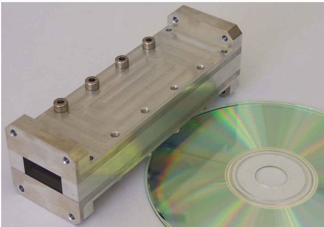
(b) Assembled filter, with compact disk for size comparison.
