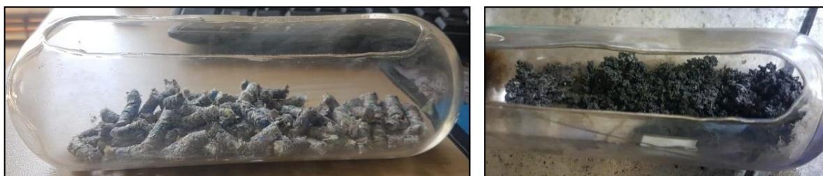
Figure B-3: The 30 g sample feed in the sample boat (left) and the char left post pyrolysis (right).
