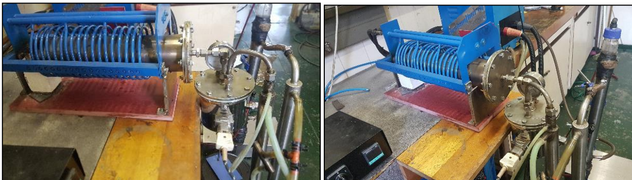
Figure B-1: The bench-scale, fixed bed reactor set-up with first collection pot, two condensers & ESP
