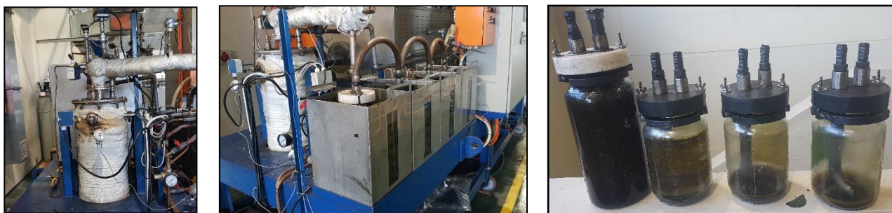
Figure B-4: The charpot (left), condensation train (middle) and condensers (right) of pilot-scale setup.
