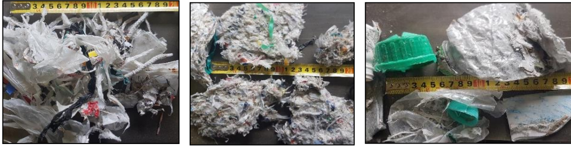
Figure A-1: Materials in pulper rejects, viz. LDPE (left), agglomerated fibres (middle), PET bottles and HDPE lids (right)
