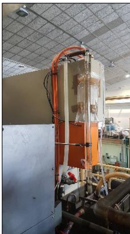
Figure B-4: The charpot (left), condensation train (middle) and condensers (right) of pilot-scale setup.
