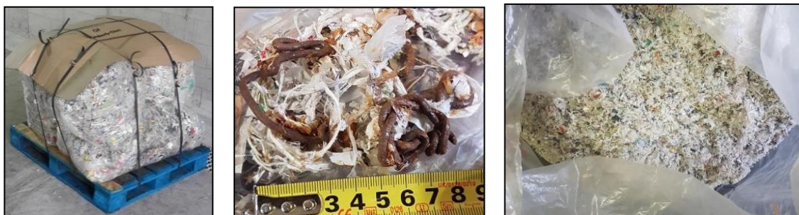
Figure 5.1: The delivered 200 kg sample (left), extracted ferrous metal (middle) and air-dried, shredded rejects (right)
