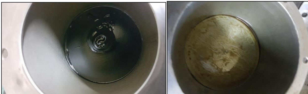
Figure B-2: The first collection pot with wax (left) and second collection pot with oil (right)
