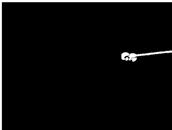
Figure 6.7: The image frame in Figure 6.6 after erosion is applied.
