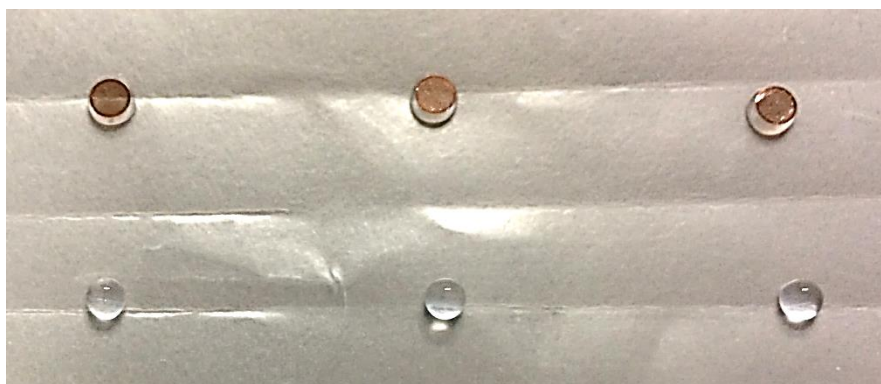
Figure 5.3. 200-mesh, carbon-coated copper TEM grids were incubated on 10 \mu l of sample for maximum proximity of grids to sample. After each step, grids were passed over distilled water, and carefully dabbed onto absorbent Whatman paper before being contrast stained with Uranyl acetate.
