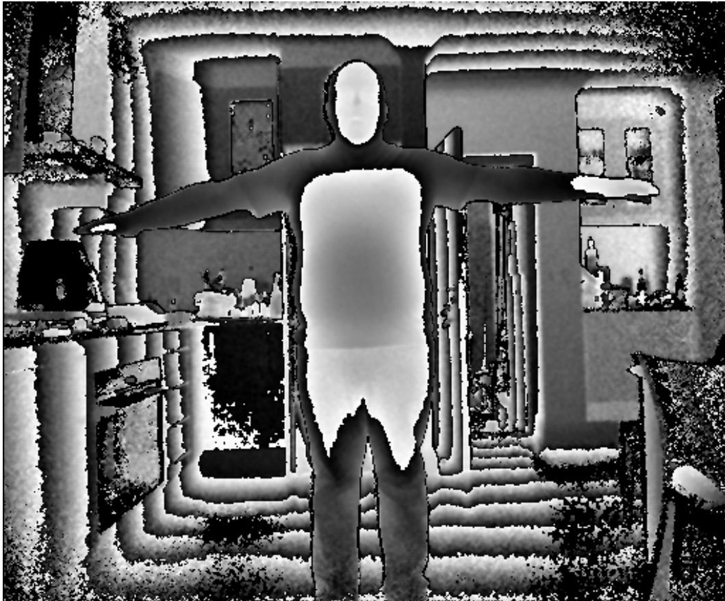
Figure 5.3: Kinect SDK Visualisation of a Kinect Depth Data Frame.
