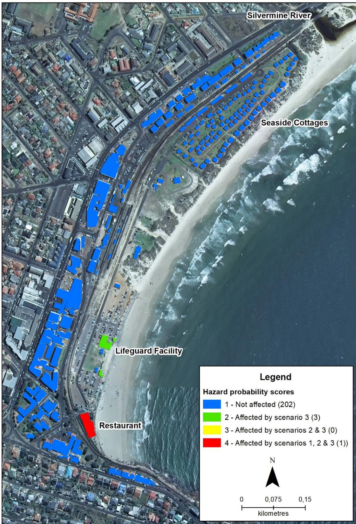
Figure 5.4 Building hazard score map of Fish Hoek (numbers in brackets give the total number of buildings per class)
