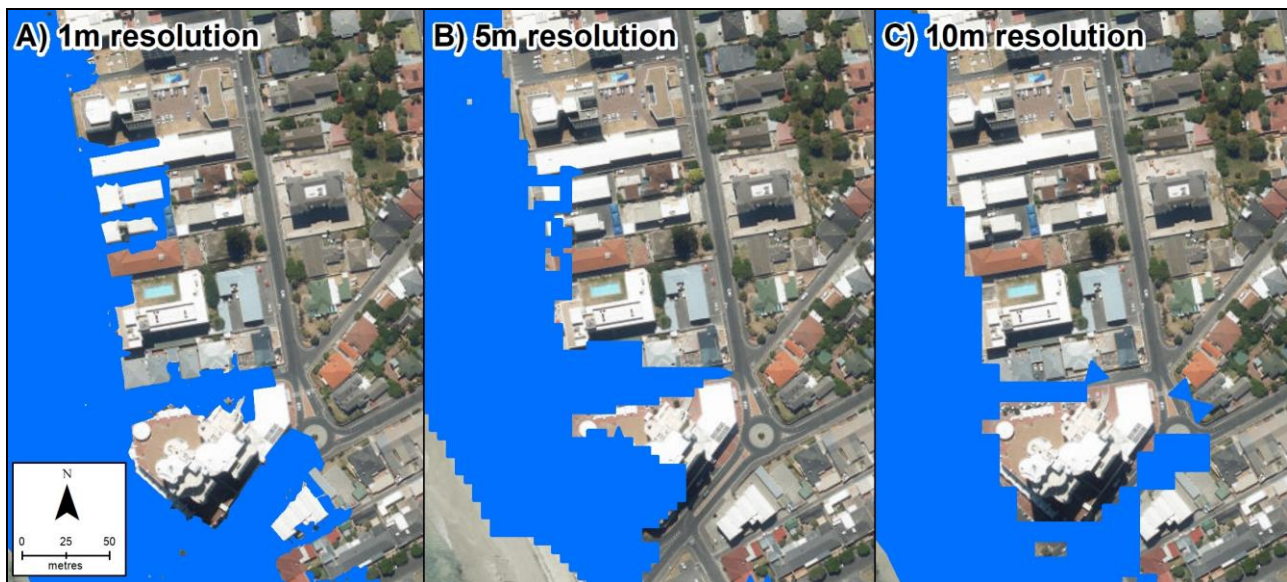
Figure 4.11 Results of the eBTM resolution test with (A) 1 m, (B) 5 m and (C) 10 m resolution DSM
