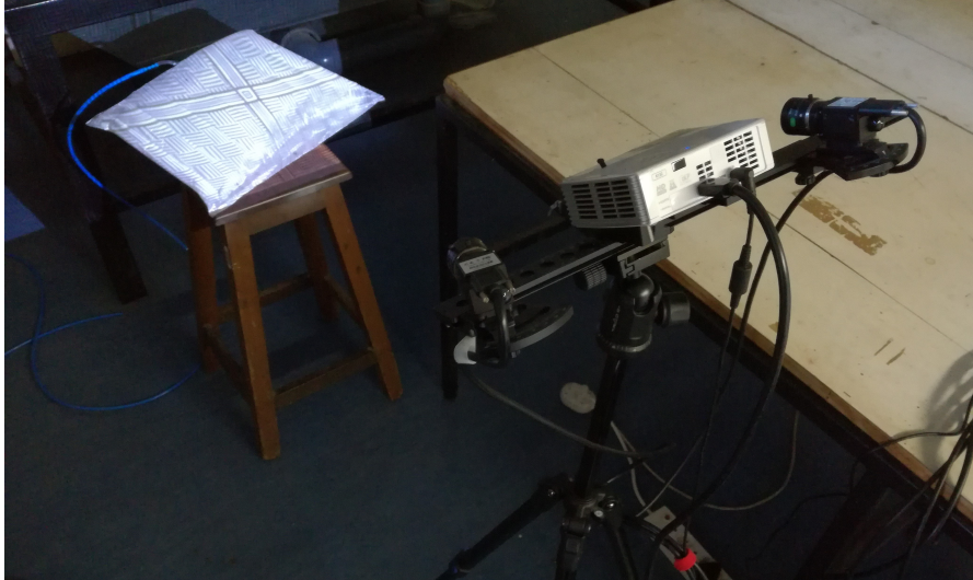
Figure 3.3: The 3D scanning setup used throughout the research, with two cameras positioned on either side of the projector
