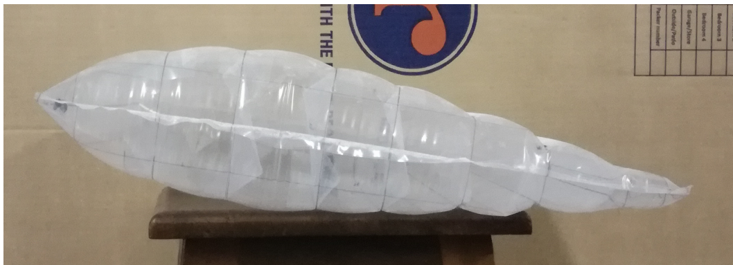
Figure 5.16: The inflated physical model of the eight cavity wing using the new construction method
