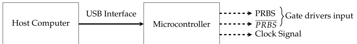
Figure 5.21: Block diagram illustration of a PRBS source
