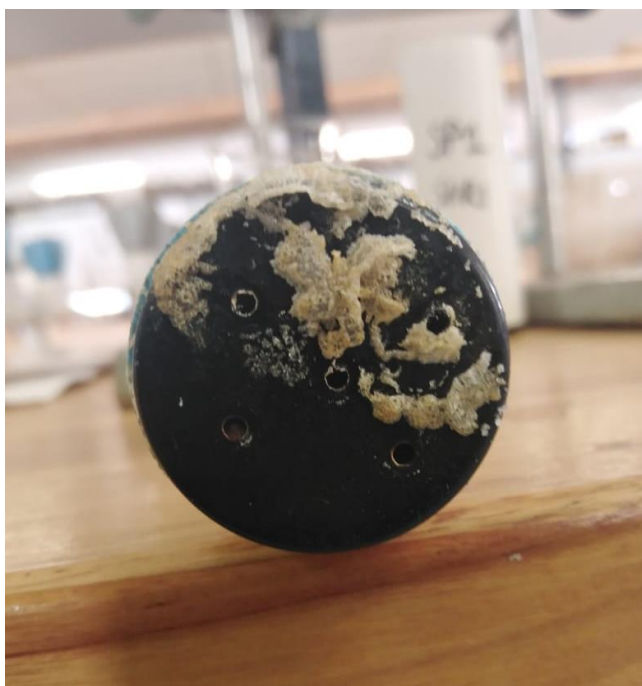
Figure 6.7: The bottom of the granite (SP1) dishwasher greywater irrigated soil when leached with rainwater.
