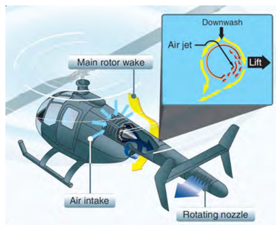
Figure 2.5: Image demonstrating the NOTAR system (Taken from [10])
