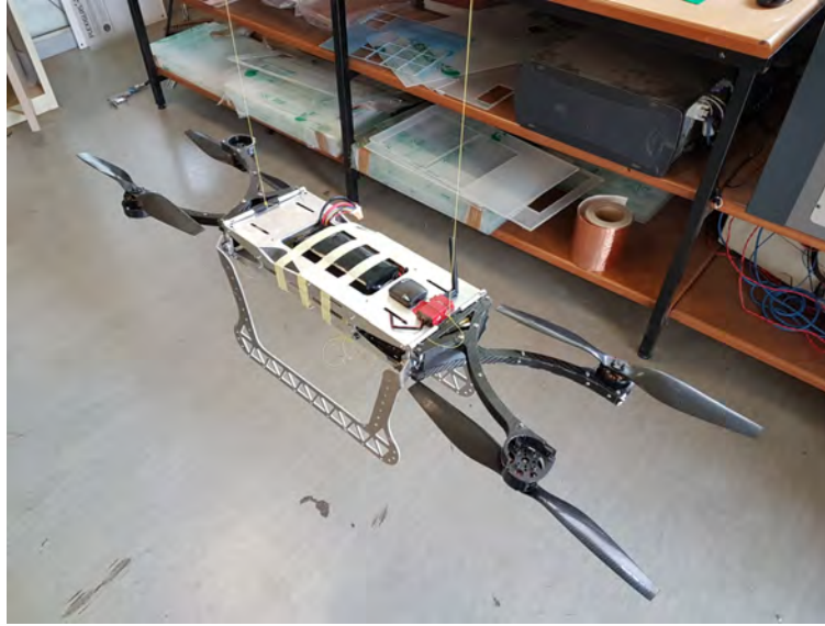
Figure 4.1: Bifilar pendulum for inertia measurement
