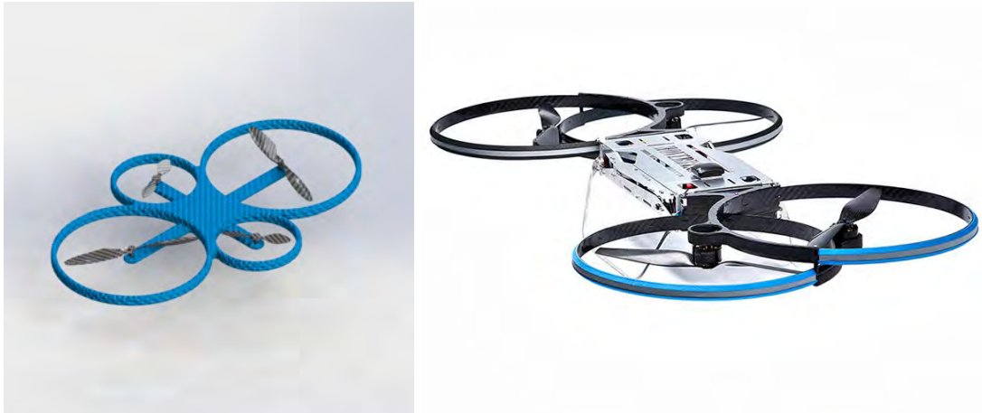
Figure 3.2: Rendering of initial concept of the unlike rotor size quadcopter (Left). Malloy Aeronautics hoverbike concept (Right) (Picture taken [41]).
