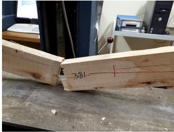
Figure 31: Bending test – brash tension failure adjacent to a finger-joint
