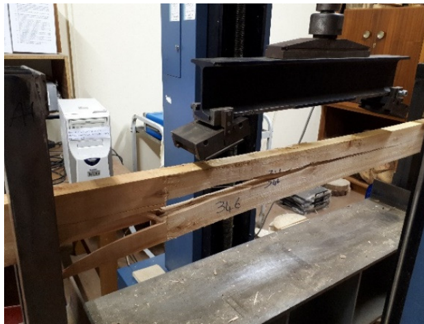
Figure 32: Bending test – diagonal tension failure originating at finger joint
