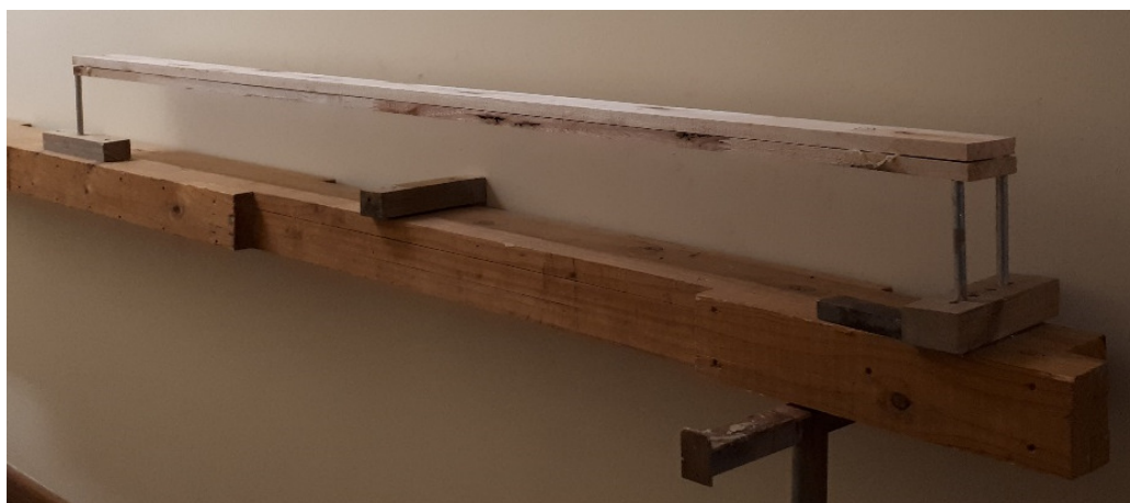
Figure 21: Warp measurement apparatus (jig)
