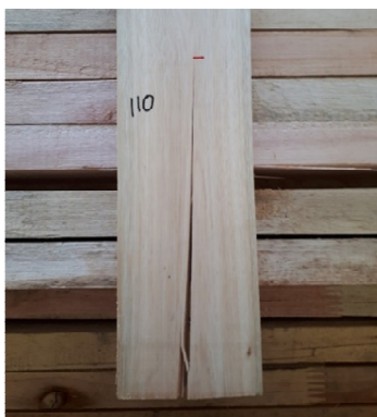
Figure 18: Surface defect marked at point of length measurement
