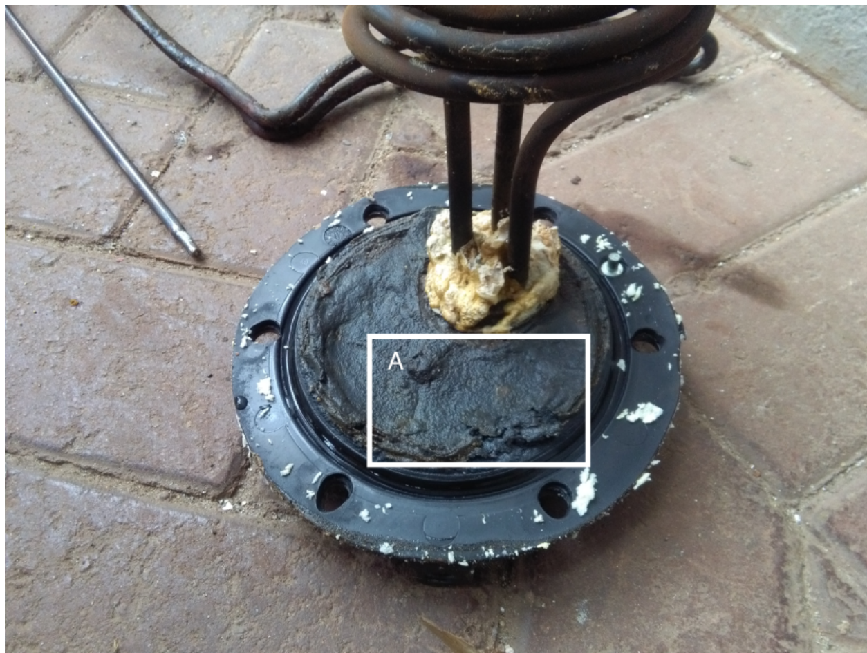
Figure A.2: Relates to section 2.4.2. Dark red-brown sludge formed against the base of the element (A), representative of the biofilm sludge sampled from the sides and elements in all EWHs within this study. Sampling was done by taking sludge scrapings in sterile petridishes or glass bottles and transporting to the lab on ice.
