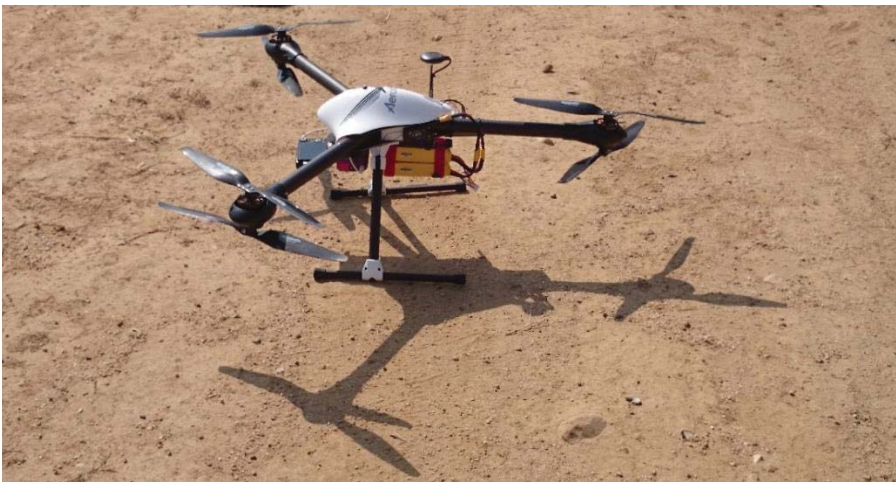
Figure 3.4 3D Robotics Y6 Trooper multirotor RPAS armed with RGB and NIR cameras.
