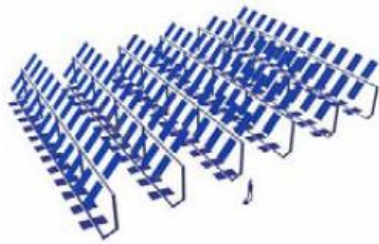
(c) Mega ganged heliostat concept by DLR (Amsbeck et al. , 2007)
