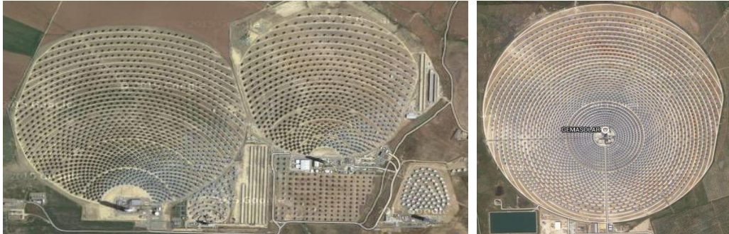
Figure 2.2: A north field used in PS-10 and PS-20 plants (Left) and a surround field used in the Gemasolar plant (Right) (Google Images, 2016).
