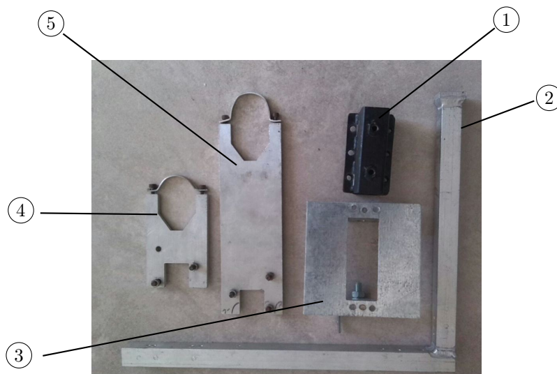
Figure C.1: Solar absolute specular reflectance measurement set up accessories. 1. Mirror frame to tracker mounting bracket. 2. Mirror frame. 3. Mirror plate. 4 and 5. CH(P)1 mounting clamp.
