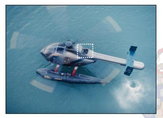
Figure 6.3 The MD 530 NOTAR with its top mounted fan intake
