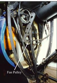
Figure 7.1 Details of the original Alouette III/CIRSTEL helicopter, showing fan intakes, space frame and fan pulley assembly
