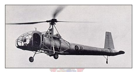
Figure 1.4 Cierva W.9, the first trials of a tail rotor-less helicopter
