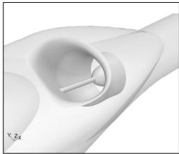
Figure 9.5 Top intake duct (fuselage displayed semi-transparent)
