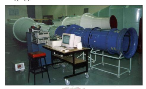
Figure A.1 The fan test-rig set up with sampling equipment
