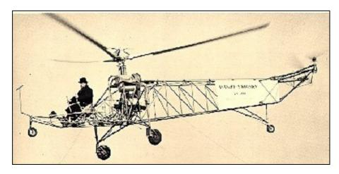
Figure 1.2 The Sikorsky VS-300, the first practical helicopter
