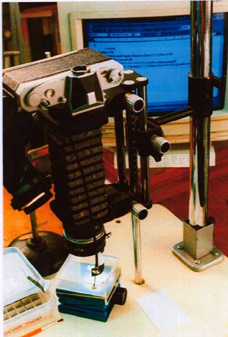
Photomacrography with Nikon PB-4 Bellows and reversed 50mm lens with E2 ring (plunger to the right). Lighting with Leitz Monlar lamp for both specimen and background; later a separate lamp was used to illuminate the background. Matte foil was used as a reflector for modelling. Focussing was done with a laboratory jack
