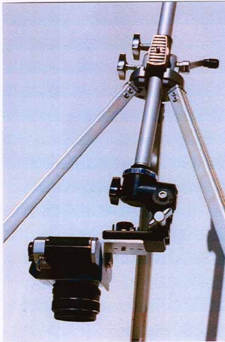
Stereophotography using 180° rotation of a tripod pan head. The convergence angle can be altered by choosing an appropriate thread in the L-piece in which to insert the camera-holding screw.
