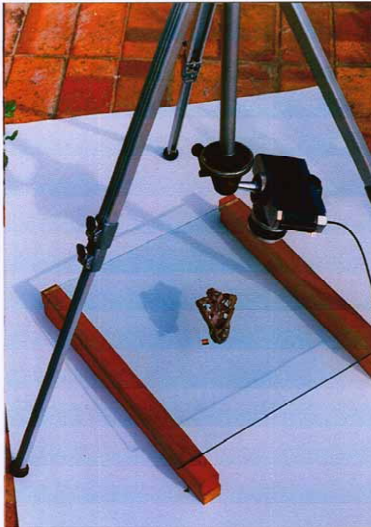
Stereophotography using 180° rotation of a rotatable tripod universal joint. The left image of the stereo-pair is being photographed (snout end of skull at the top). The specimen is placed on a sheet of glass to allow the shadow to fall outside the frame of the photograph.
