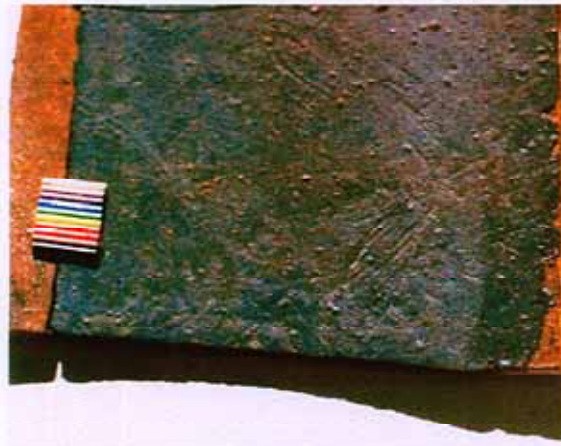
Portion of a polyester replica made on the underside of a slab (natural cast). Strips of Masonite were taped around the part with tracks (fish trails) to make a shallow well for the resin. The resin had black pigment added, and 600 Corundum grit to simulate the texture (settling of the grit during setting was not a problem).
