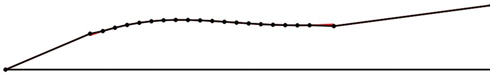
Fig. 4.6. 2-D profile of the ideal and linear approximated smoothed Klopfenstein taper in a conical line without a central conical to coaxial transition. The red part is the ideal taper, and the black part the linear approximated smooth taper.
