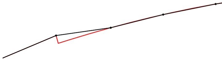
Fig. 4.7. 2-D profile showing the smoothed edge of the conical line Klopfenstein taper. The red part is the ideal taper, and the black part the linear approximated smooth taper.
