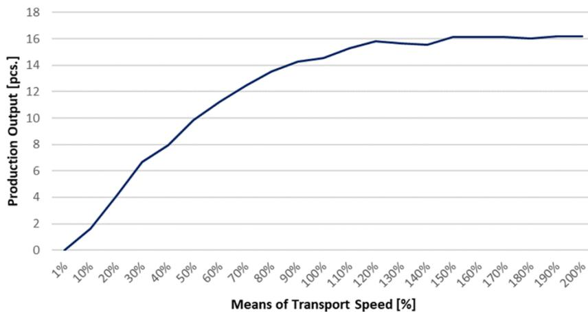
Figure 6-8: Influence of the means of transport speed on production output
