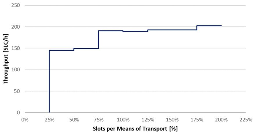
Figure 6-10: Influence of the means of transport capacity on throughput
