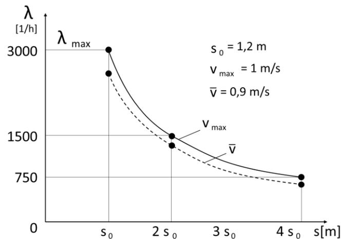
Figure 3-1: Correlation of throughput and distance on a material flow route according to Arnold and Furmans (2005, p. 12)
