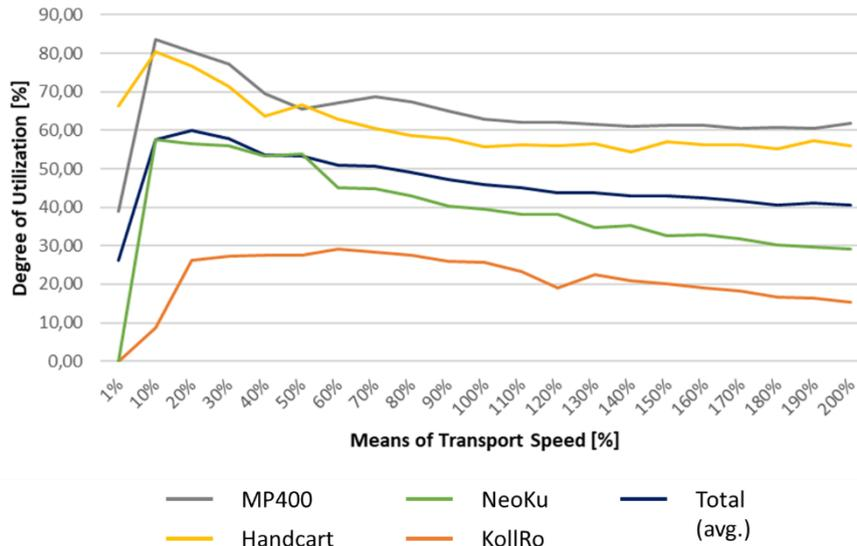
Figure 6-9: Influence of the means of transport speed on the degree of utilisation of the means of transport
