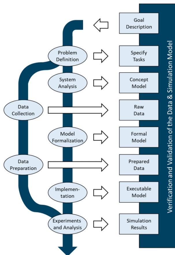
Figure 1-2: Process model of simulation according to Rabe et al. (2008, p. 5)
