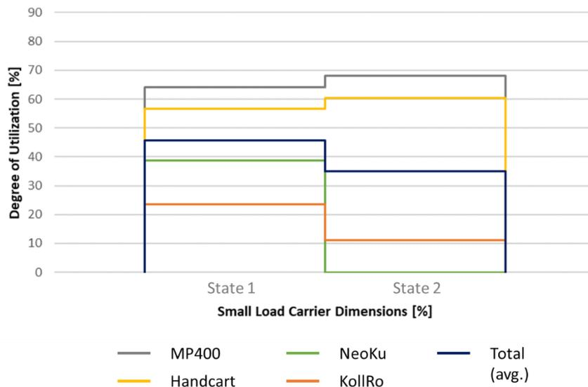
Figure 6-15: Influence of the product dimensions on the degree of utilisation of the means of transport
