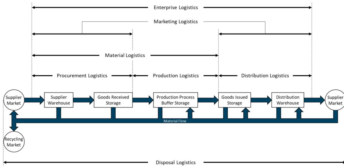
Figure 2-3: Functional differentiation of logistics systems according to Pfohl (2010, p. 19)
