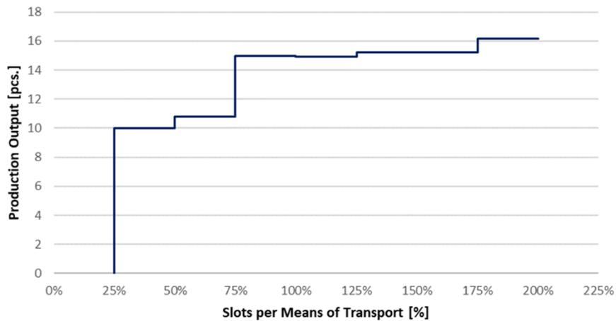
Figure 6-11: Influence of the means of transport capacity on production output
