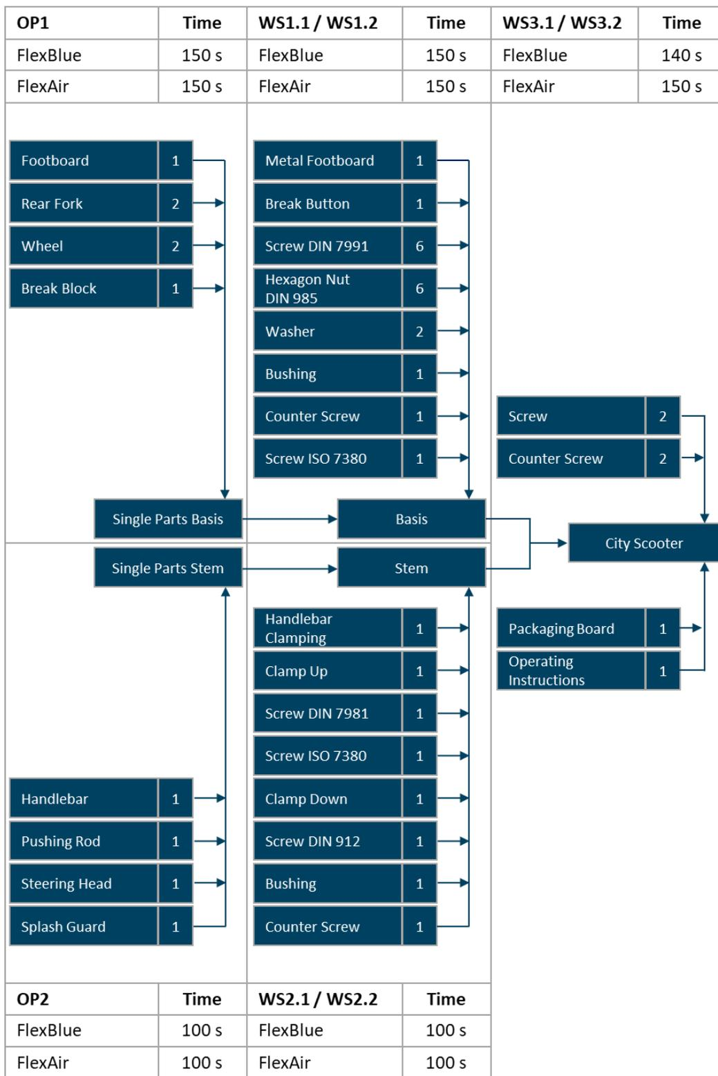
Figure 2-18: Assembly plan of the two city scooters according to Große Erdmann (2020, p. 37)
