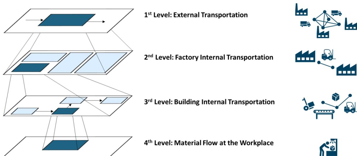
Figure 2-6: Hierarchical levels of material flows according to Bullinger and Lung (1994, p. 5)
