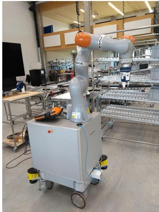
*Figure C-3: NeoKu with its Kuka iiwa*
