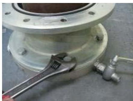
**Figure 59: Bolting of the pipe extension**
