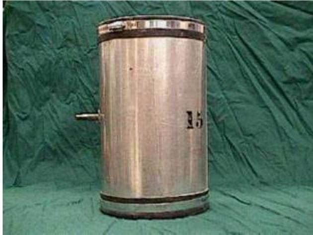
**Figure 21: Texas triaxial cell** (Crockford et al, 2002)
