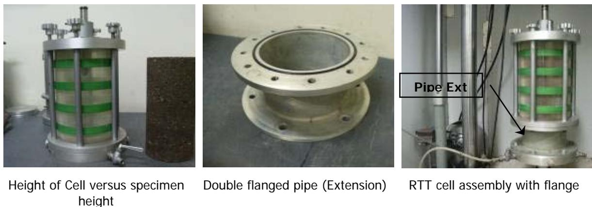
**Figure 58: Height extension of the RTT**
