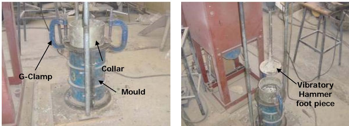
**Figure 57: Photos showing extension collar attachment on mould**
