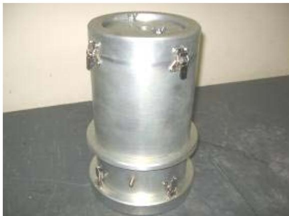
(vii) Place the cell in the hydraulic loading frame; adjust actuator position until visual contact is made with the loading ram.
