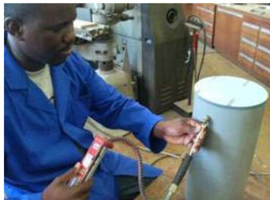
**Figure 39: Trial cell pressure testing**
