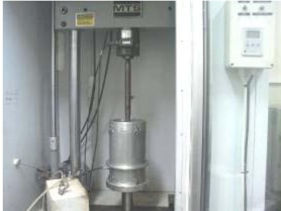
(ix) Set monotonic test parameters on the MTS controller including displacement rate of strain (2.1%), full-scale for the loading (10.0V = 98.1 kN) and half-scale for the displacement (10.0V = 40mm)
