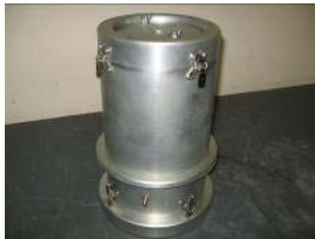
**Figure 47: Assembled STT cell**
