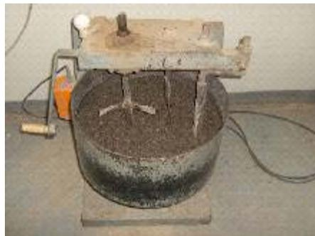
**Figure 53: Laboratory vertical shaft drum mixer**
