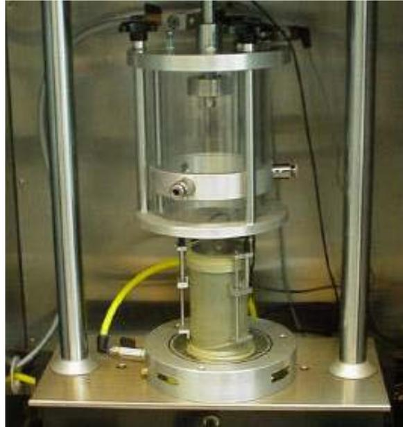
**Figure 28: The RaTT Cell** (Crockford et al 2002)
