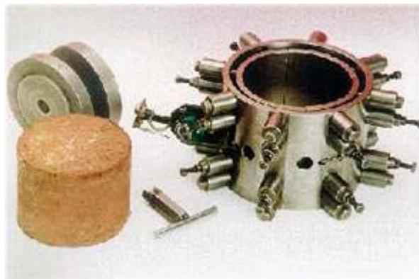
**Figure 27: K-Mould apparatus** (Dynatest, 2008)
