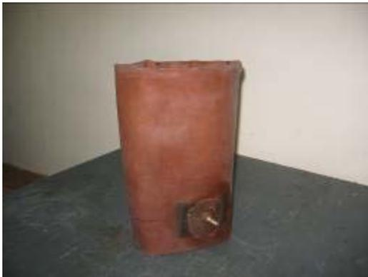
Figure 42: Valve fitted on tube
