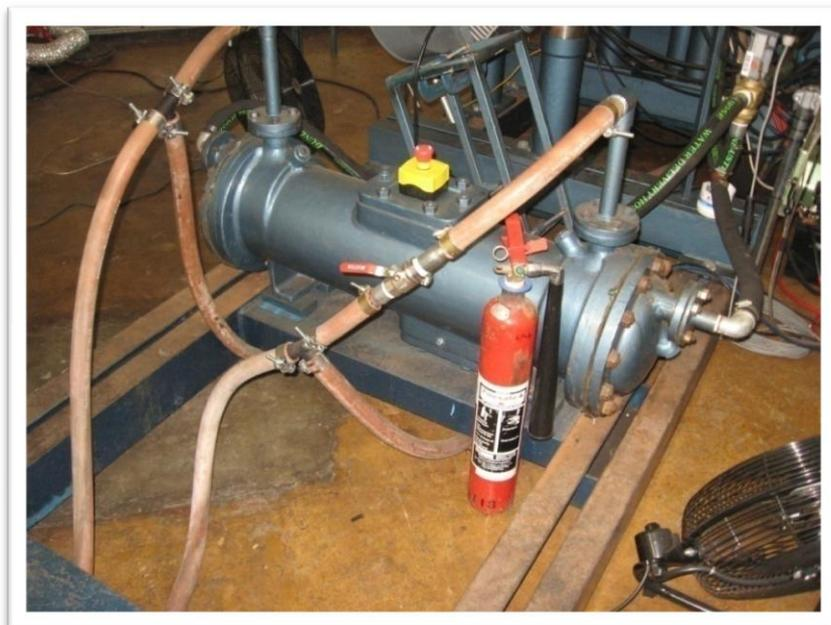
FIGURE 64 - SHELL AND TUBE HEAT EXCHANGER
