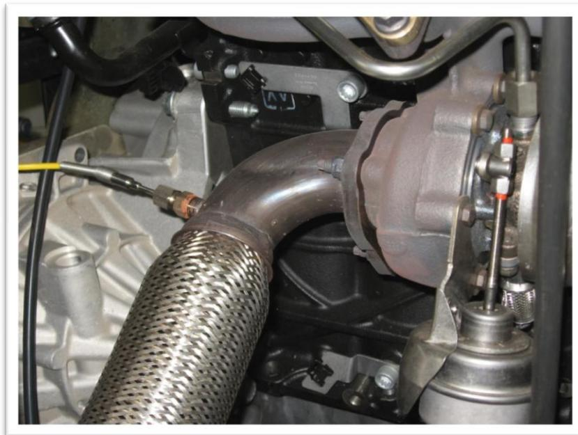
FIGURE 60 - EXHAUST THERMOCOUPLE INSTALLATION
