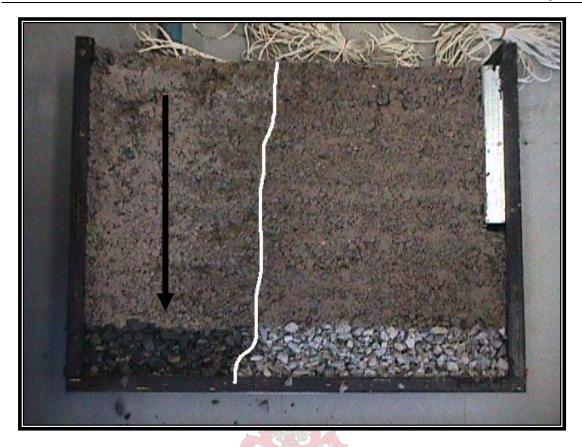
Figure 6.1 Wetting front for 30% fines, 8% water, 0 mA, 7 days test
