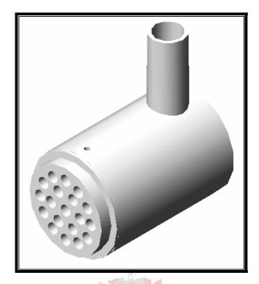
3-Dimensional anode compartment (One-dimensional test)
