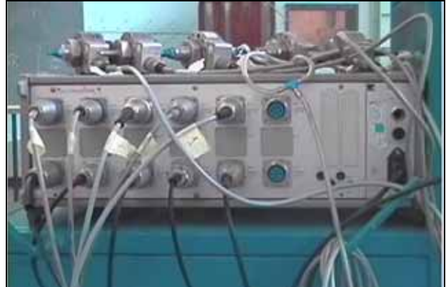
Figure 4.28. HBM bridge amplifier back showing input and output plugs.
