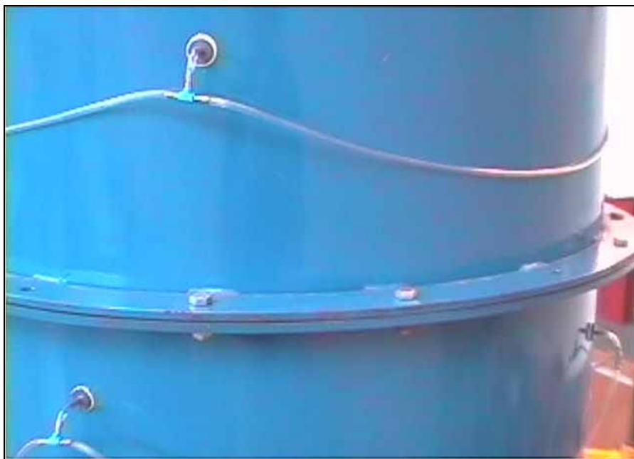
Figure 4.19. Pressure tapping points on turbine exit pipe.
