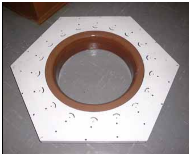
Figure 4.7. Upper ring showing the ducting leading into the diffuser.
