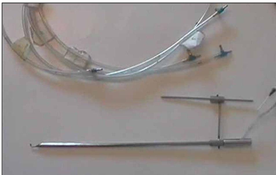
Figure 4.24. Five-hole probe with piping to be connected to pressure transducers.
