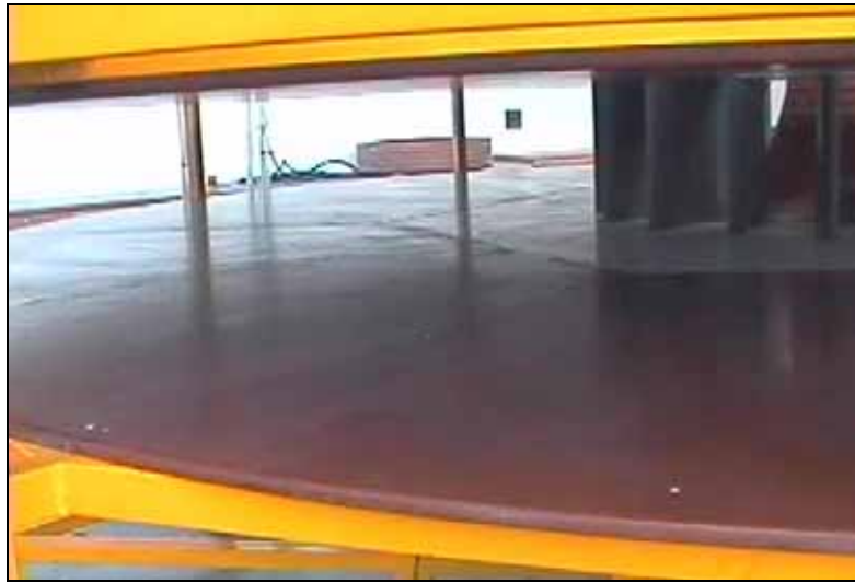
Figure 4.8. Inlet ducting leading into inlet guide vanes.
