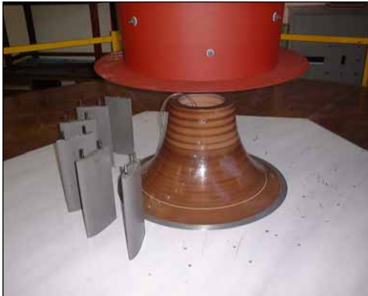
Figure 4.6. Moulded inlet guide vanes in position around central cone.
