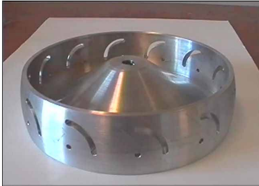
Figure 4.10. Turbine hub showing spherical shape and grooves for adjustable stagger angles.
