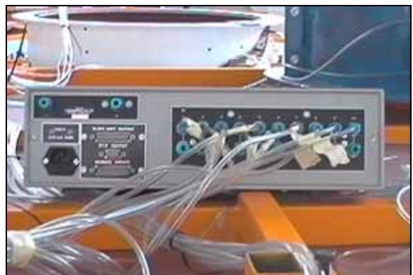
Figure 4.30. Pressure switching box back panel with multiple inputs.
