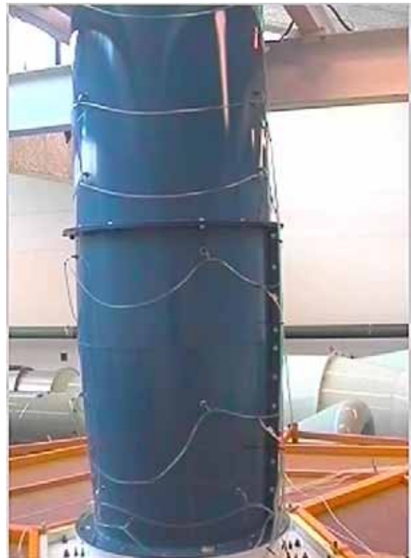
Figure 4.26. Picture of pressure tapping points and connecting pipes.
