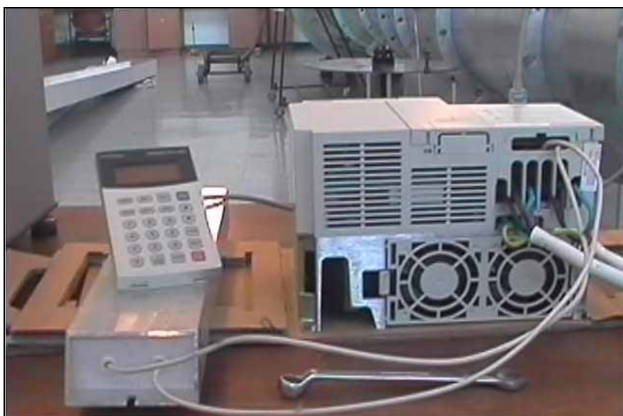
Figure 4.13. Generator coupled to variable speed drive with brake resistor.
