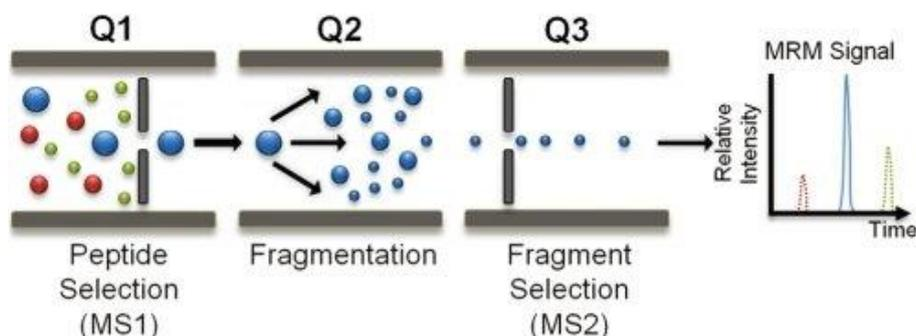
Figure 1.7: Multiple Reaction Monitoring Mass Spectrometry (MRM-MS). MRM-MS utilises the signal of selected MS2 fragment ions for quantification. It is commonly conducted on a triple-quadrupole instrument: Q1 selects a precursor ion, Q2 fragments the precursor ion and Q3 selects a specific fragment ion for the detector <sup>(139)</sup>
