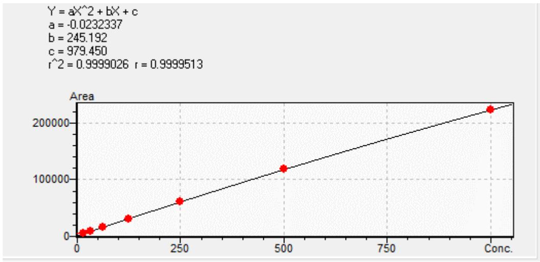
Calibration curve of acetylcholine from 31.3 - 1000 ng/mL with a quadratic regression and 1/C weighting
