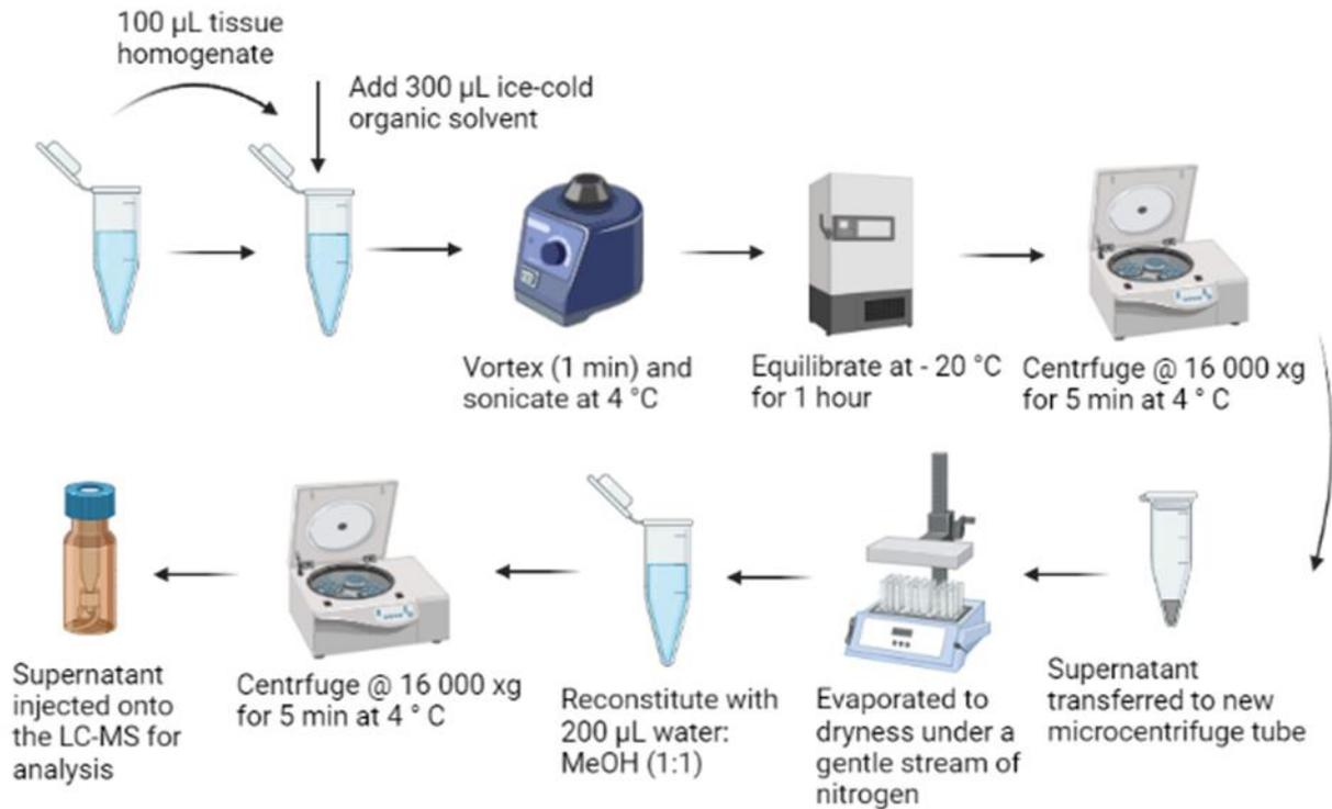
Figure 2.4: The protein precipitation extraction method development. Image created using Biorender
