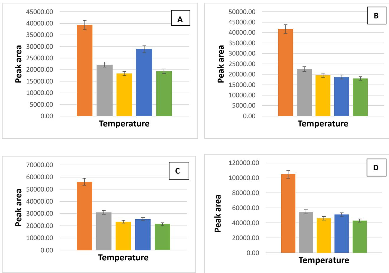
Figure 2.2: The relationship between peak area and heating block temperature (°C) for acetylcholine (A), dopamine (B), gamma-aminobutyric acid (C) and serotonin (D). (Orange - 250 °C; grey - 300 °C; yellow - 350 °C; blue - 400 °C and green - 450 °C)
