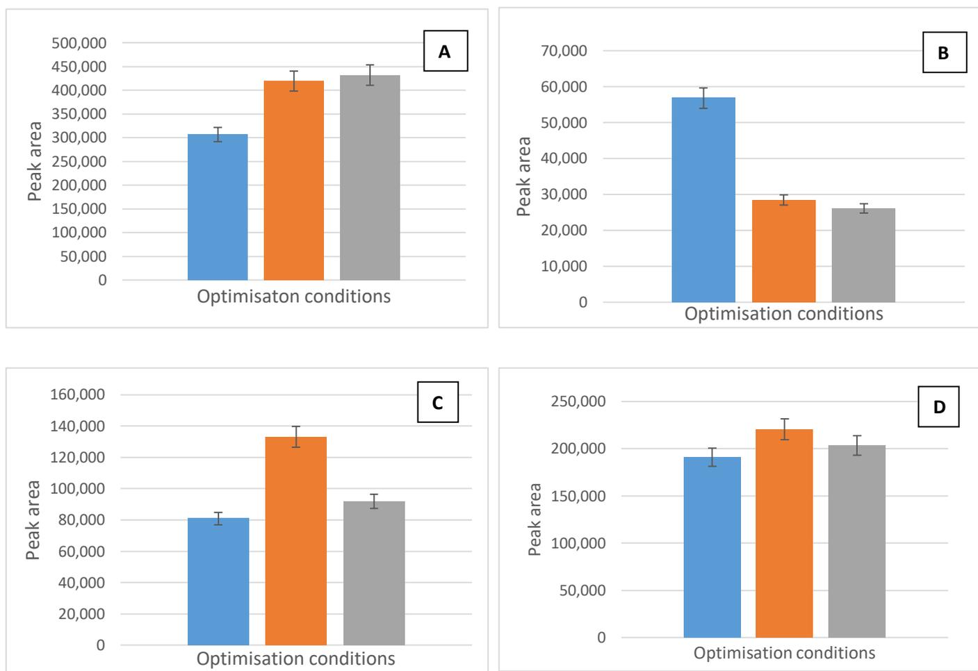
Figure 2.6: The relationship between the average peak area of serotonin (A), acetylcholine (B), dopamine (C) and gamma-aminobutyric acid (D) and various extraction optimisation conditions. (Blue - supernatant injected directly onto LC-MS; orange - supernatant eluted through HLB cartridges, concentrated under nitrogen and reconstituted in MeOH:water (1:1, v/v) and grey - supernatant concentrated under nitrogen and reconstituted in MeOH:water (9:1, v/v))
