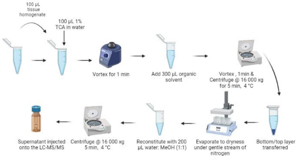
Figure 2.3: The liquid-liquid extraction method development. Image created using Biorender
