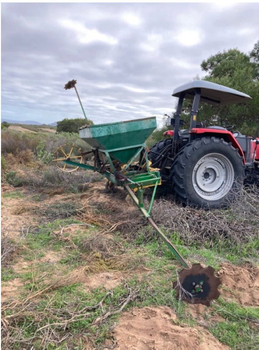
Figure 2.9: Plant Ripper With a Fertiliser Tank Attached
