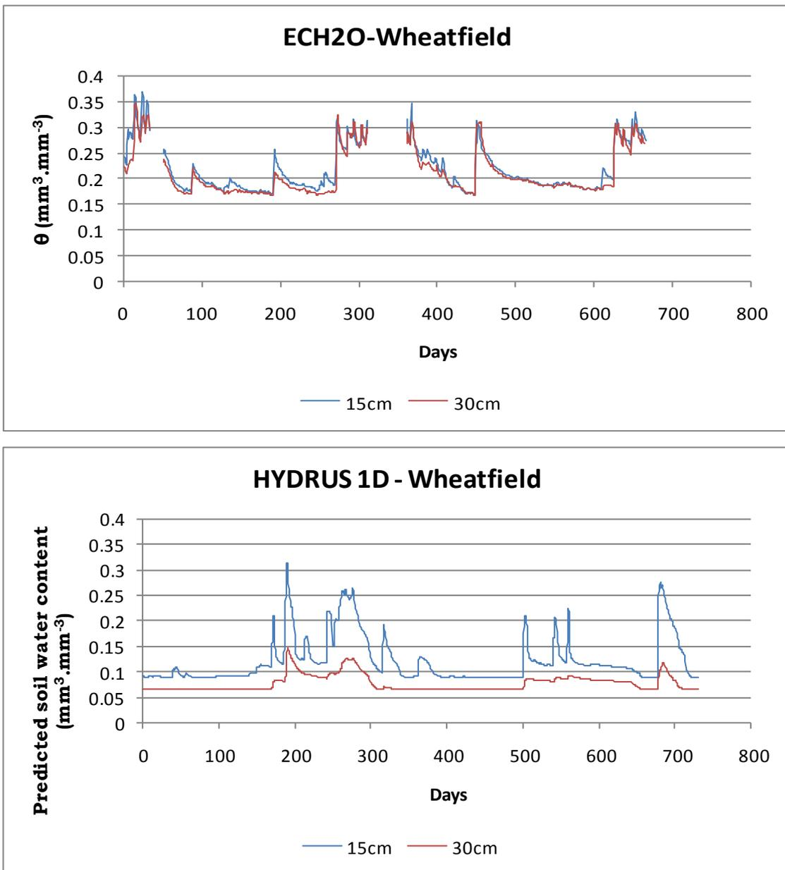
**Figure 5.05** ECH2O sensor field measured soil water content compared to predicted soil water content at 15cm and 30cm depths for the wheatfield for the period 17 August 2008 – 16 August 2010.
