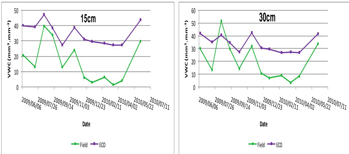
**Figure 5.04** Graphs indicating the comparison of field (gravimetric soil water content) and ECH2O sensor measurements for (a) the Renosterveld and (b) the wheatfield for selected depths.
