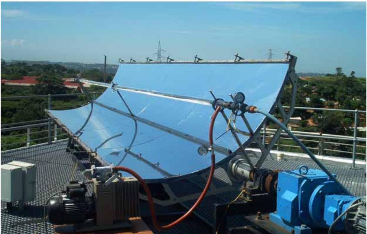
**Figure 3.3** PTSC with glass-shielded receiver during operation and vacuum pump visible in foreground
