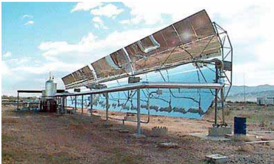
**Figure 2.2** Parabolic trough test loop, Plataforma Solar de Almería (www.psa.es, 2004)
