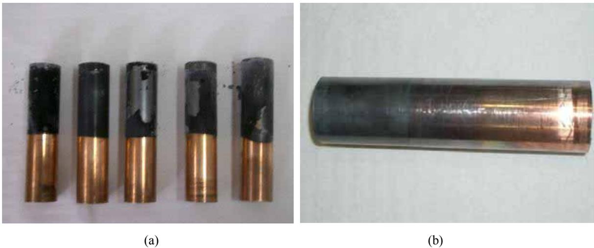
**Figure A.18** (a) Samples of tube with  $\text{Cu}_2\text{S}$  coating obtained after exposure to  $\text{NH}_4\text{S}$  for (left to right) 20 s, 40 s, 60 s, 120 s and 5 min (b)  $\text{CuO}$  surface coating showing blue-black finish
