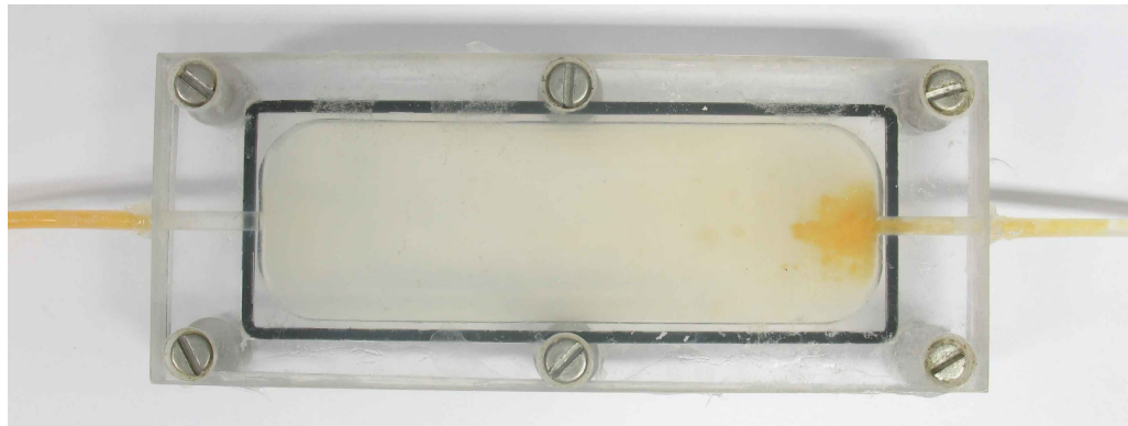
FIG. 3.1. Biofilm growth of isolate YO64 in a flat-plate reactor (channel size: 100 mm × 30 mm × 6 mm) of 36 h post-inoculation in enriched Anacker and Ordal's medium.
