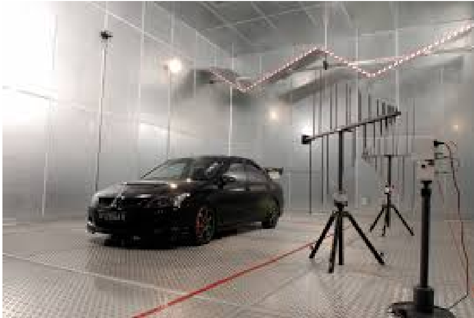
Figure 2.10: Reverberation chamber for shielding effectiveness measurement [24].
