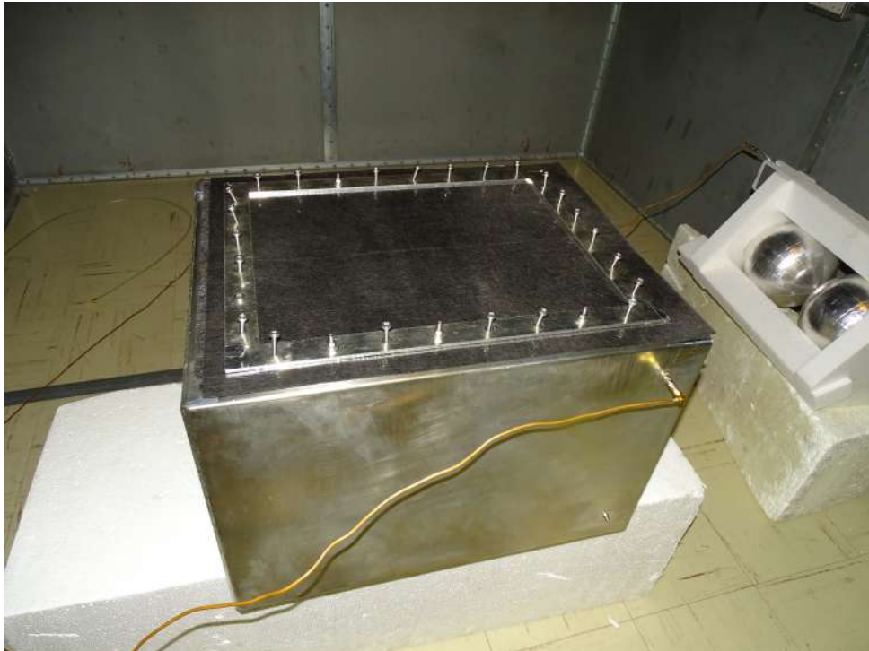
Figure 4.9: Photograph of the nested chamber with material placed directly in contact with the nested chamber surface. No measures taken to minimize RF leakages.
