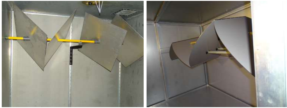
Figure 2.11: Different stirrer designs as used in the two different chambers in this study. The shape and size of the stirrer used affect the measurement significantly.
