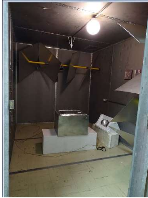
Figure 3.2: The reverberation chamber as used in the majority of work in this thesis. This is set up as per the nested chamber method
