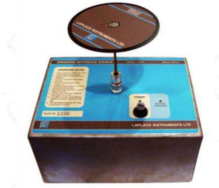
Figure A.2: A photograph of a comb generator used for time domain measurements.
