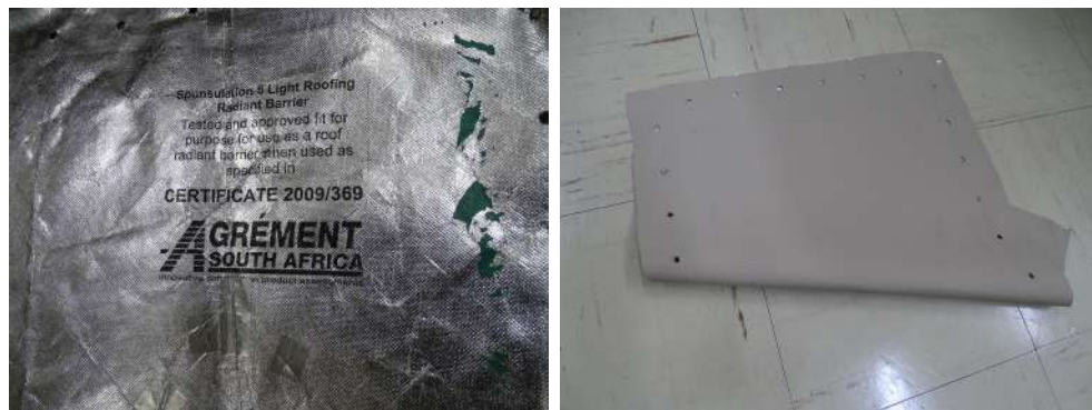
Figure 3.16: (a) Spunsulation 5 roofing radiant barrier material (b) Silver ripstop material
