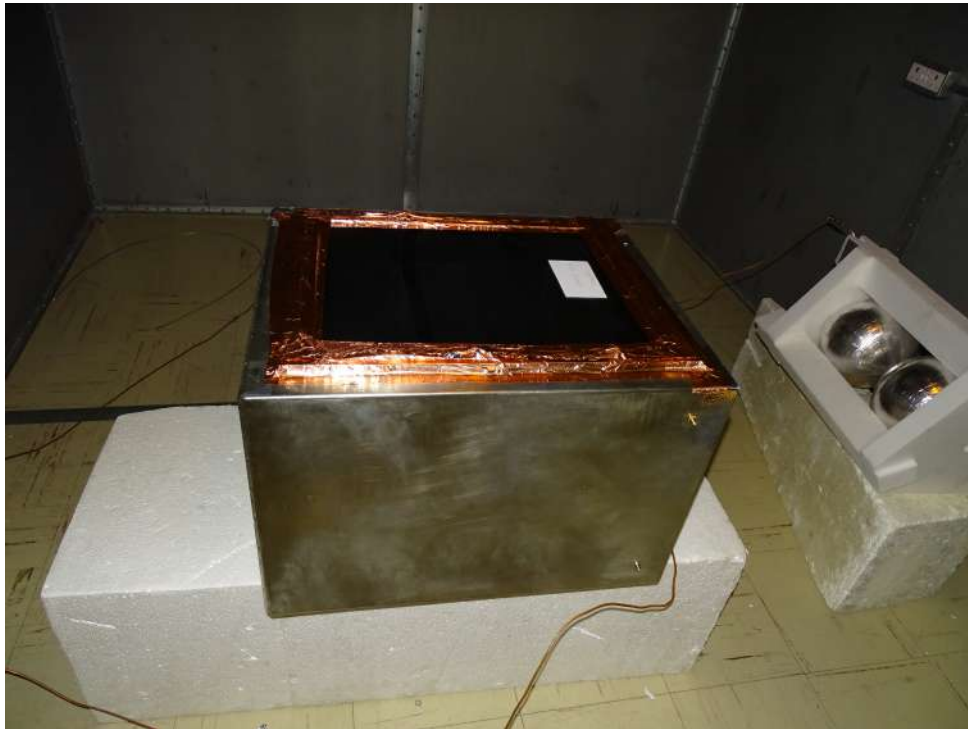
Figure 4.11: Photograph of the nested chamber sealed with copper tape on the edges and over the bolts, to prevent RF energy leakage.
