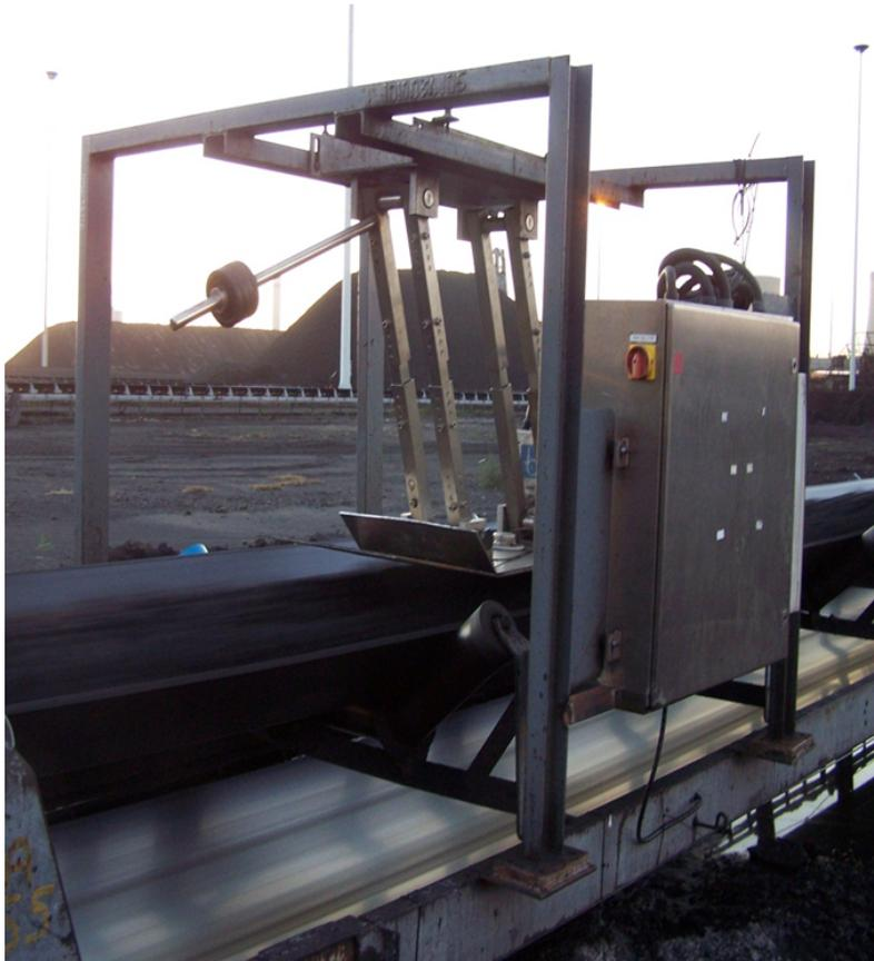
Figure 2: An image of an X-Ray Fluorescence analyser (XRF).
