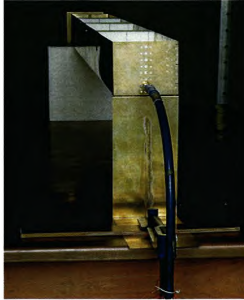
Figure 5.2: Photograph of the back end of a cable tray connected to port two of an ANA with a co-axial cable.
