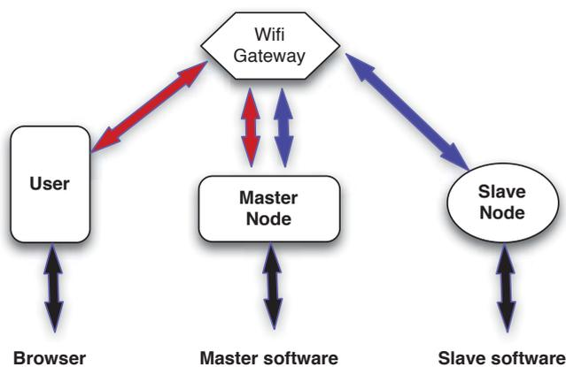
Fig. 4. Functional Software Layout (note. Only one slave is depicted in this figure).
