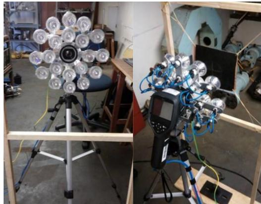
Figure B.3: Front-on heating setup in operation
