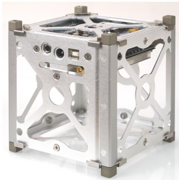
**Figure 2.1** – The Skeleton of a CubeSat
