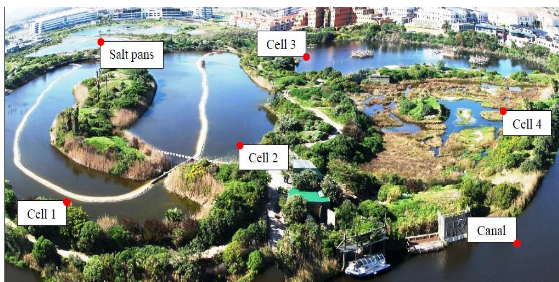
Figure 15: Panoramic view of the constructed wetland's four treatment cells
