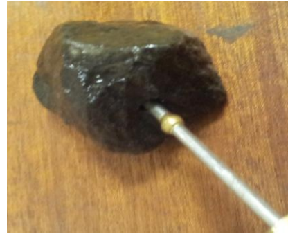
Figure 4.5: Rock temperature measurement technique
