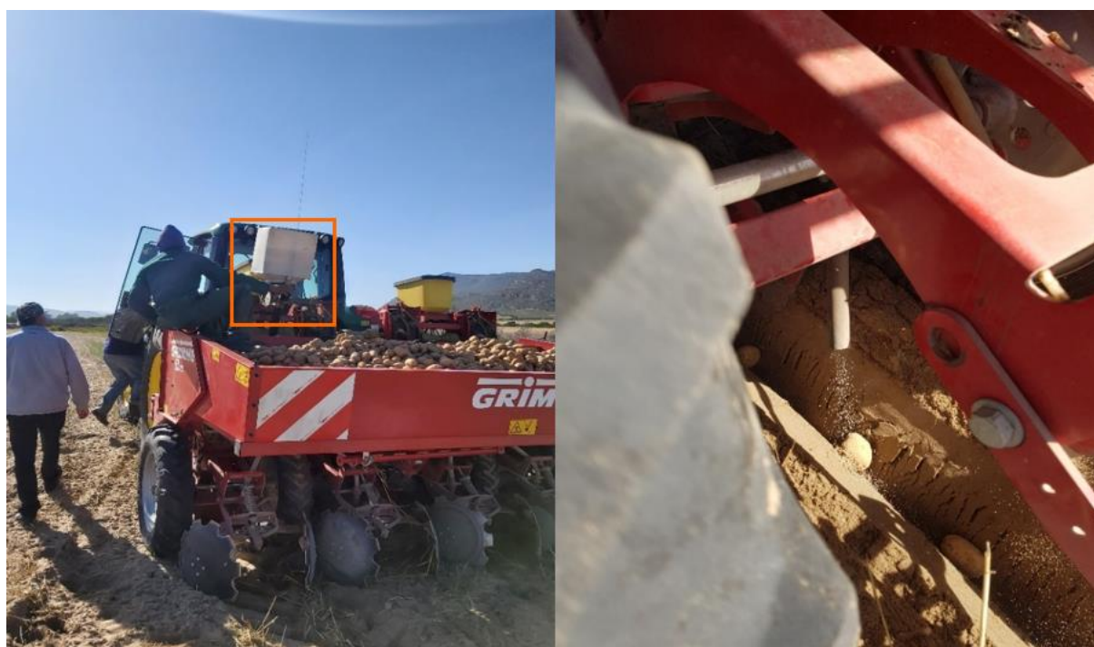
Figure 3.2 The planter with the applicator, indicated by the orange block (left), and the Zeba™ being applied in the planting furrow along with the tubers (right).
