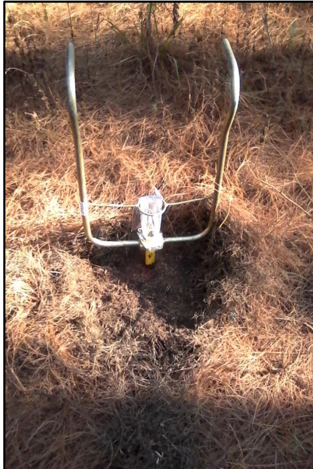
Figure 3.13: Beater auger used for sampling of the top soil.
