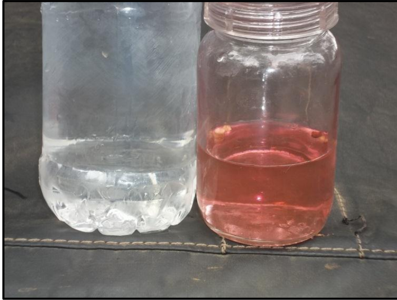
Figure 3.17: Discoloration of the tetrazolium solution on the right hand side indicate that the cambium sample is still alive.
