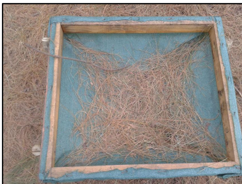
Figure 3.15: Illustration of the littertraps built and used for this study to calculate monthly litterfall rates.
