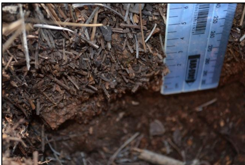
Figure 3.14: Determining FF depth with a ruler after exposing the whole FF profile using a shovel.
