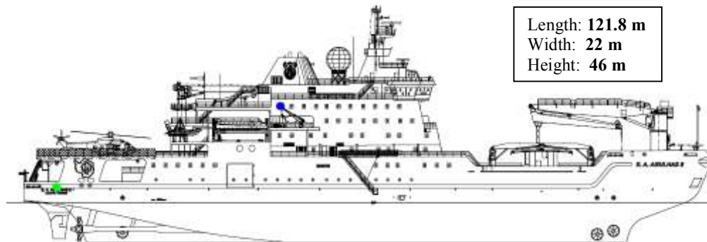
Figure 3.1: Location of the accelerometers on Deck 3 and Deck 8
