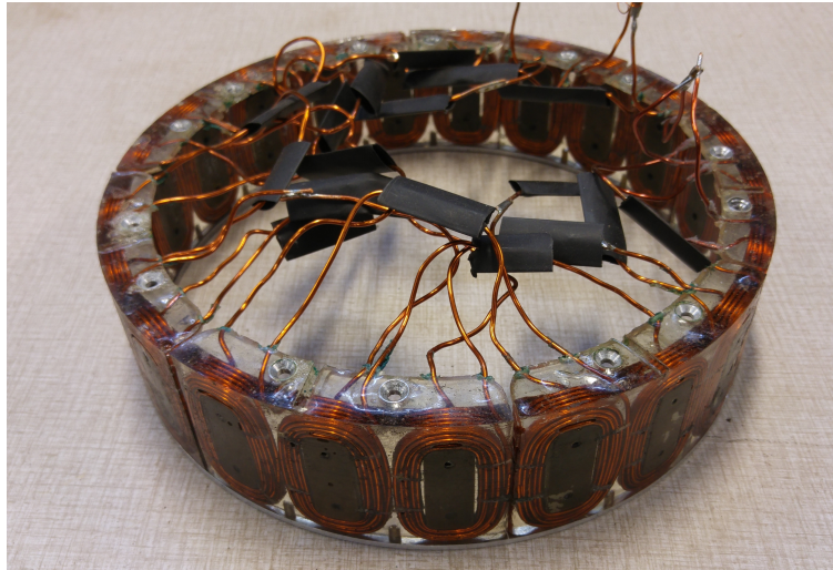
Figure 6.5: The 1.6 mm coils used to test eddy effects.
