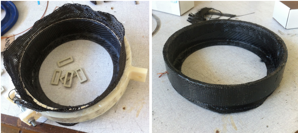
Figure 4.8: Inner rim magnets with CFRP layer.
