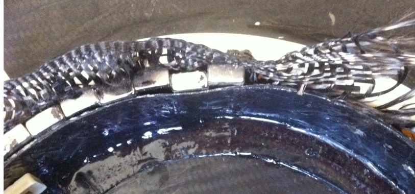
Figure 4.9: CF deformation during magnet mounting.
