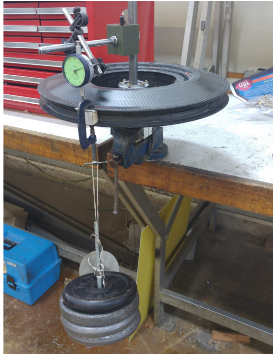
Figure 6.19: Testing deflection of the rotor under lateral load.
